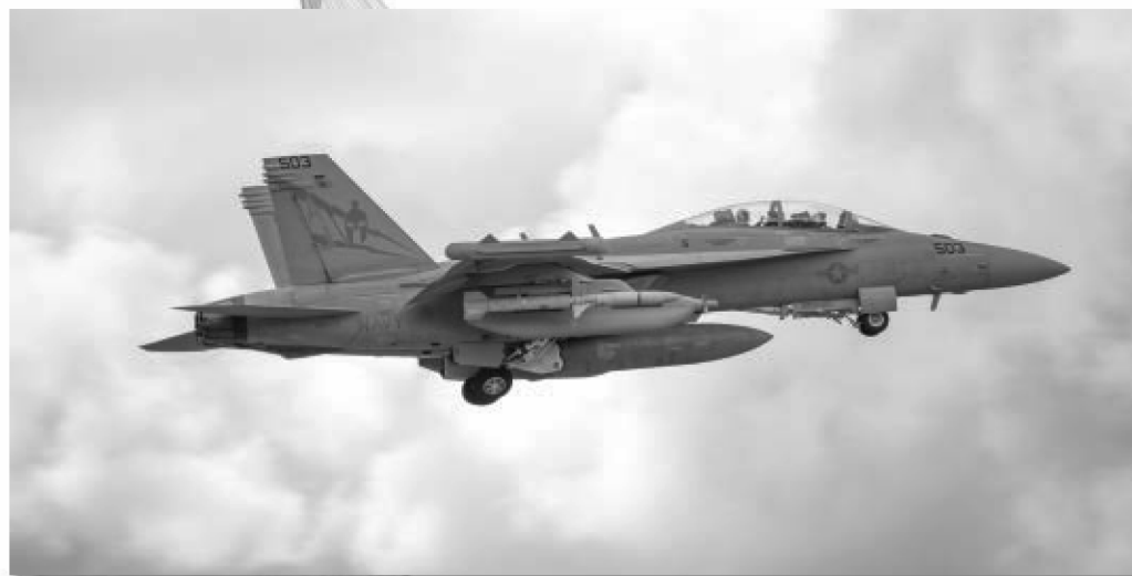
The EA-18G's ALQ-99 pods rely on TWTs to generate the power needed to perform its support jamming mission.
