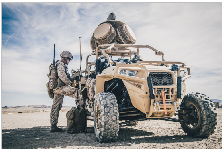
Programming a counter-unmanned aircraft system on a Light Marine Air Defense Integrated System
